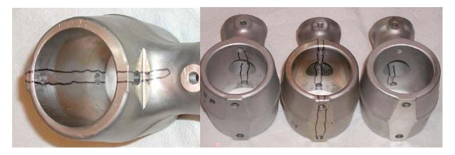
17. When reassembling the horn assembly onto the torque tube, do not torque the through bolts to 140 inch/pounds as these are in shear, not tension. The proper torque is 65 inch/pounds for the through bolts.
