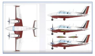
wing root fillets (top and bottom), the rudder balance weight, the stabilator repairs, the wiring of new navigation LED lamps, and wing surface patches
