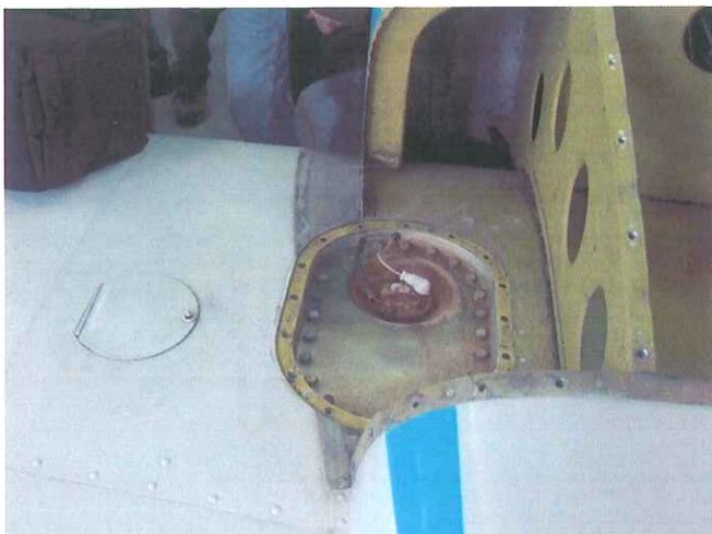
A common spot for corrosion to start
